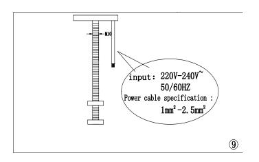
2. Install the lamp body into the derrick and lock the lamp with nuts; Connect the lighting cable to the ceiling power input cable with a waterproof junction box.
